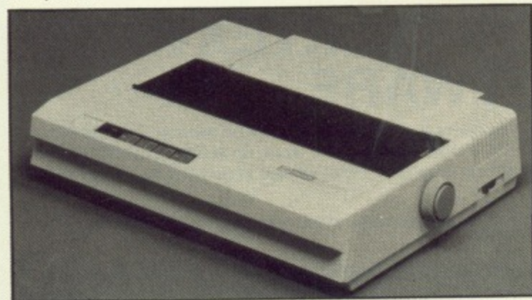
MP165 80 column 165 CPS draft 26 NLQ, tractor and friction feed, IBM and Epson compatible £169
